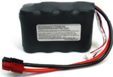
The 4S2P battery pack has a nominal voltage of 13.2 volts and a total capacity of 4.6 Ah. Capable enough to power a 100 W rig for longer periods of operation than our other packs, and will allow you to run your lower-powered rig for many hours.
