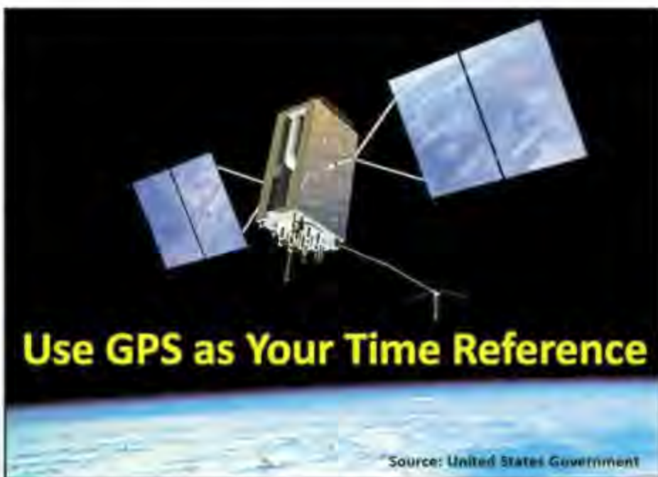
Figure 1. With a simple receiver and inexpensive software, you can use GPS satellites to keep your computer clock accurate from any place where you can see the sky.
