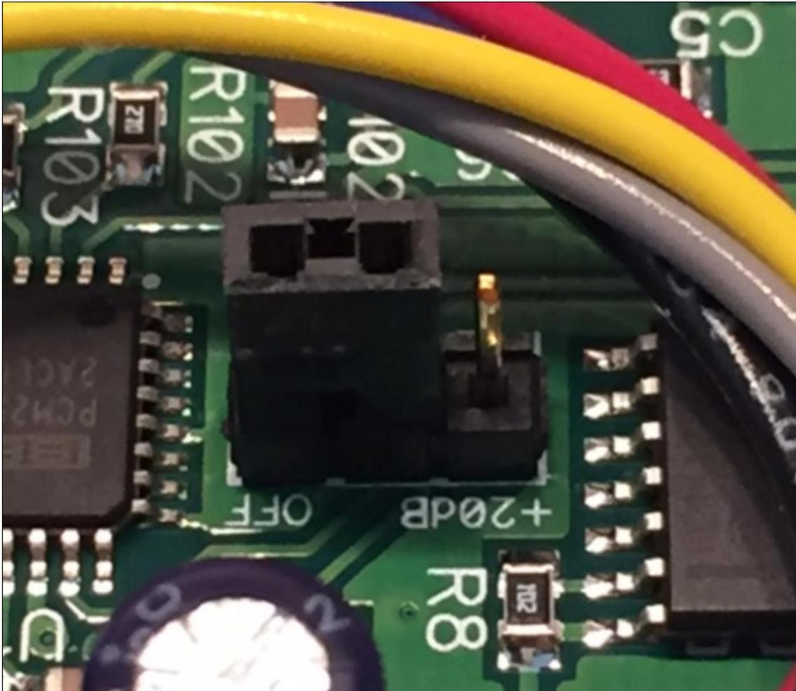
**Figure 3. Photograph of +20dB and OFF Position and Jumper**
