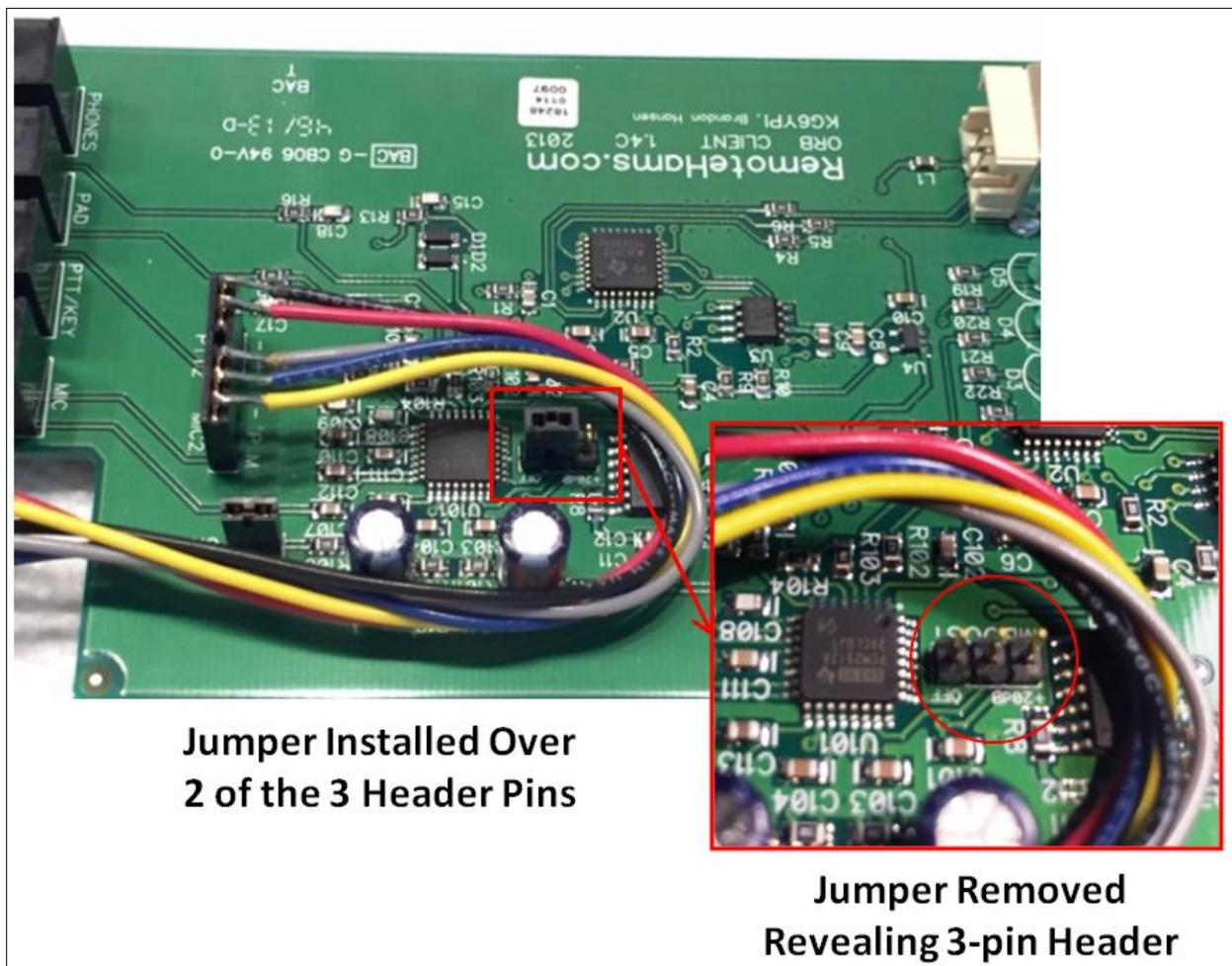
*Figure 2. Photograph of ORB Control Device Circuit Board Assembly*
