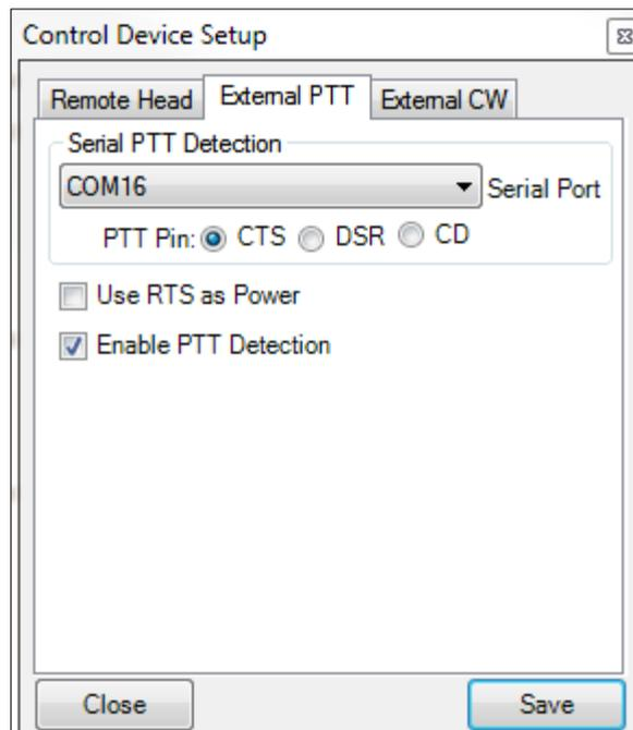
**Figure 6. Photograph of PTT Interface Panel**
