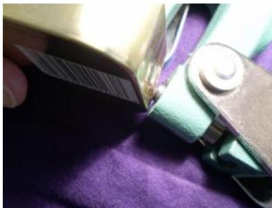
Screw the 1/4" die in the bottom jaw, and insert the 1/4" punch in the top (movable) jaw.
