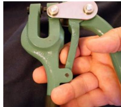
***The key to accurate punching is to bring the tin to the punch and nestle the dimple on the point of the punch before squeezing.***
