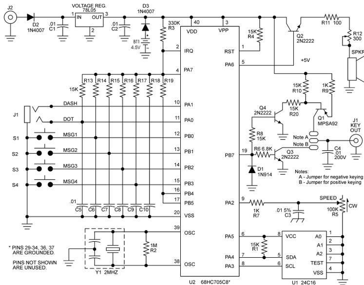
Note: For negative keyer rigs, the internal jumper goes to the outside two pins of the header, for solid state rigs use the two inside pins of the three pin header.
