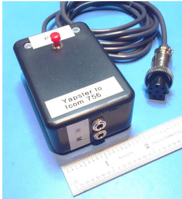
Figure 2. Prototype AIU For Icom 746/756 Radios Using Foster 8-pin Jacks
